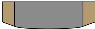
Flat Across Top and Slightly Rounded Comfort Fit with Square (contoured) Edges
